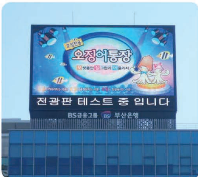
부산은행(부산) (W)14,5×(H)8,75m / 15,625mm Pitch
