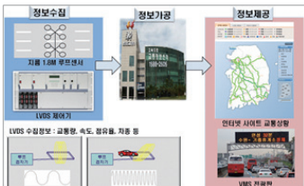
VDS(Vehicle Detection System)
